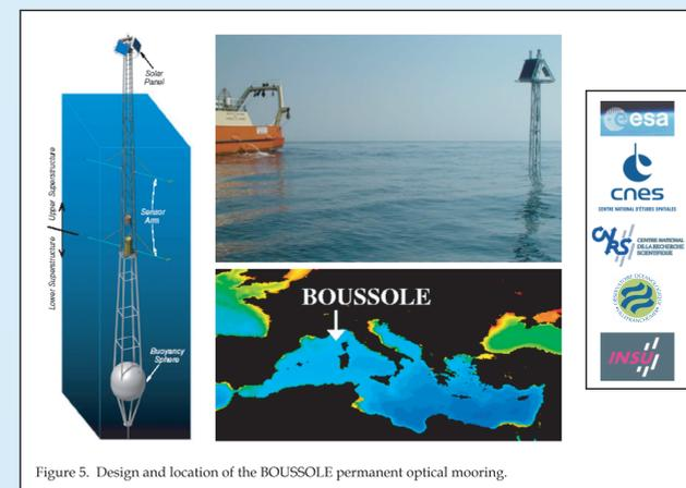
Figure 5. Design and location of the BOUSSOLE permanent optical mooring.
