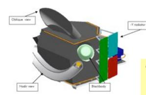
Conical scanning imaging radiometer with dual view capability:
