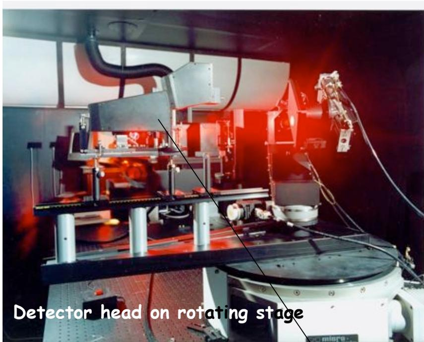
Detector head on rotating stage
