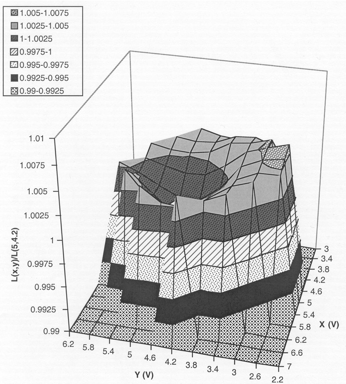
**Fig. 27.** Spatial variability of the spectral radiance  $L(487.1)$  viewed normal to the plane of the exit aperture of the GSFC sphere, as measured with the SXR on 9 Sept 1994. The values are plotted relative to the radiance at the center of the exit aperture, i.e., at  $(x, y) = (5.0 \text{ V}, 4.2 \text{ V})$ . Variability of similar shapes and amplitudes was measured at 411.5 nm and 774.8 nm.
