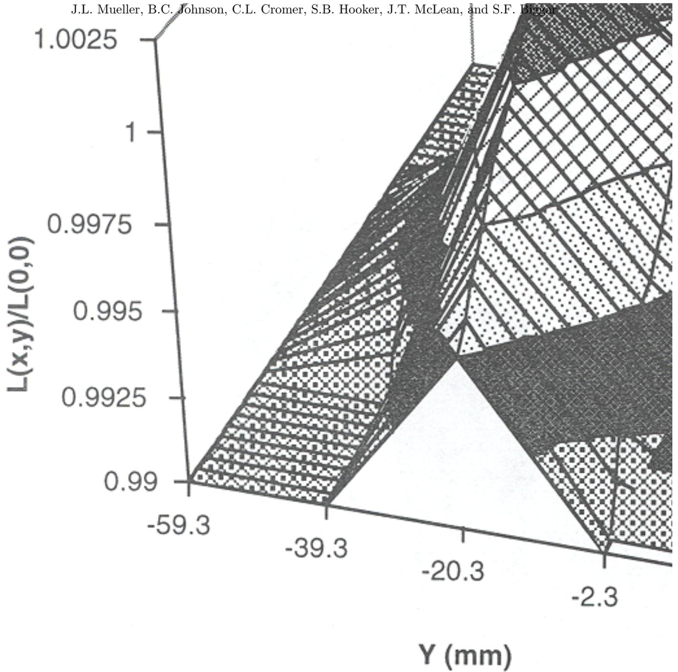
**Fig. 28.** Spatial variability of the spectral radiance  $L(531.9)$ , viewed normal to the plane of the exit aperture of the CHORS sphere, as measured with the CXR on 12 and 13 Sept 1994, just prior to SIRREX-3. The values are plotted relative to the radiance measured at the center of the exit aperture, i.e., at  $(x, y) = (0 \text{ mm}, 0 \text{ mm})$ .
