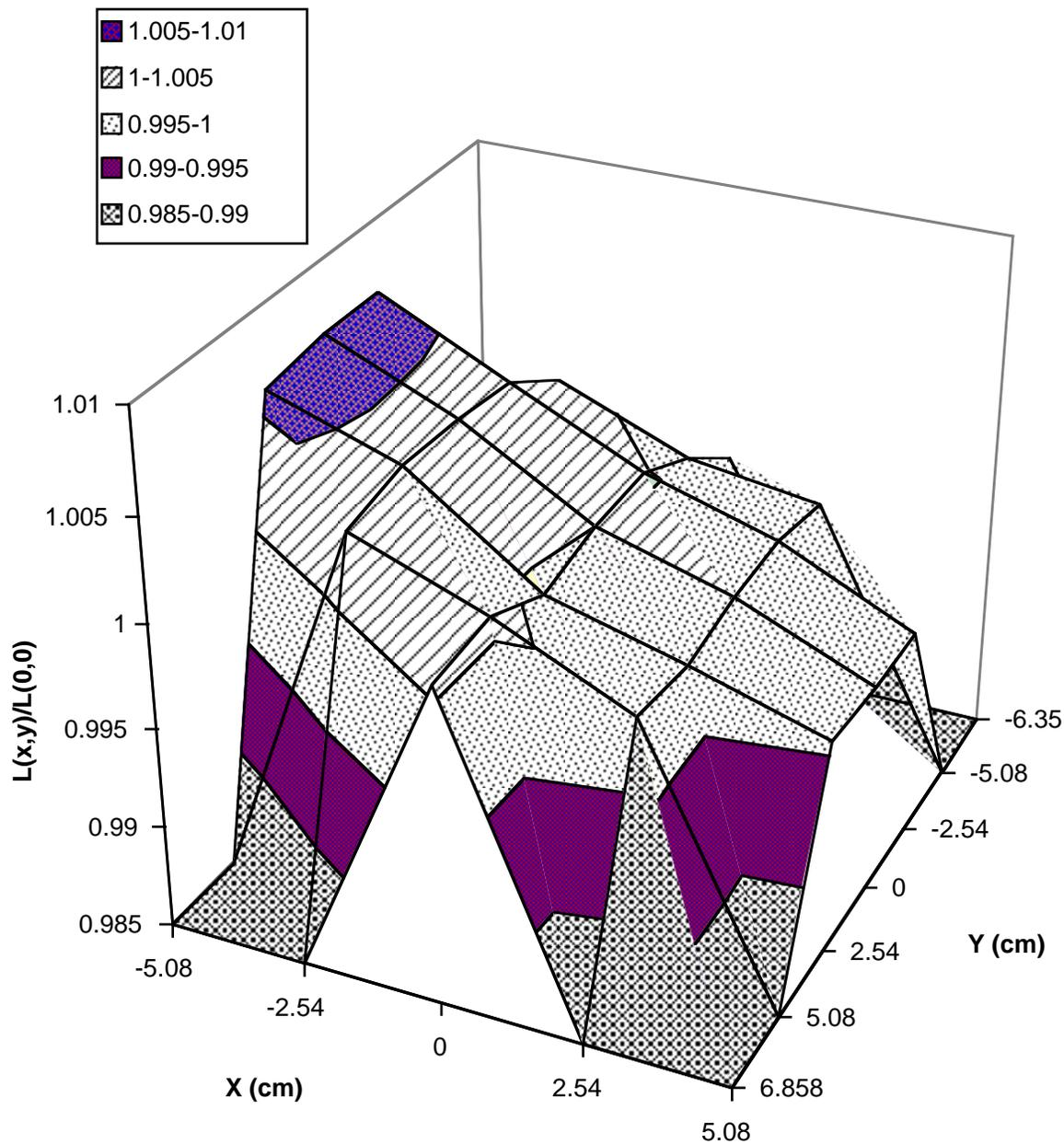
**Fig. 29.** Spatial variability of the spectral radiance  $L(487.1)$ , viewed normal to the plane of the exit aperture of the UCSB sphere, as measured with the SXR during SIRREX-3. The values are plotted relative to the radiance measured at the center of the exit aperture, i.e., at  $(x, y) = (0 \text{ cm}, 0 \text{ cm})$ . Note that unlike Figs. 27 and 28, the  $x$  and  $y$  axes have been plotted here in reverse orientation.
