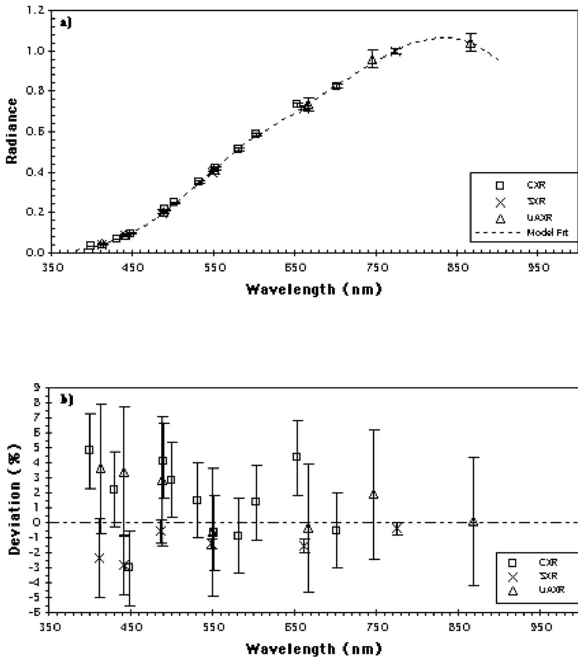
**Fig. 19.** a) Average spectral radiance in units of  $\mu\text{W}/(\text{cm}^2 \text{sr nm})$  of the BSI sphere as measured with the SXR, the UAXR, and the CXR, shown with the model fit to these data. b) Results from panel a) with respect to the model fit and the uncertainties, calculated as described in the text. The quantity plotted (see legend) is the CXR, SXR, or UAXR data minus the model fit, normalized to the model fit.
