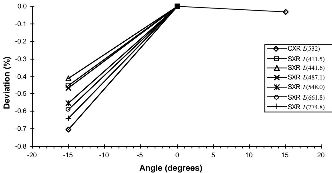
**Fig. 31.** Lambertian quality (angular uniformity of radiance) of the CHORS sphere, measured within 15° of the normal to the center of the plane of the exit aperture using the SXR (all wavelengths) and the CXR (531.9 nm only). The quantity plotted is the spectral radiance at a particular viewing angle minus the spectral radiance at normal incidence, normalized to the normal incidence value, for the indicated measurement wavelengths of the SXR and the CXR.
