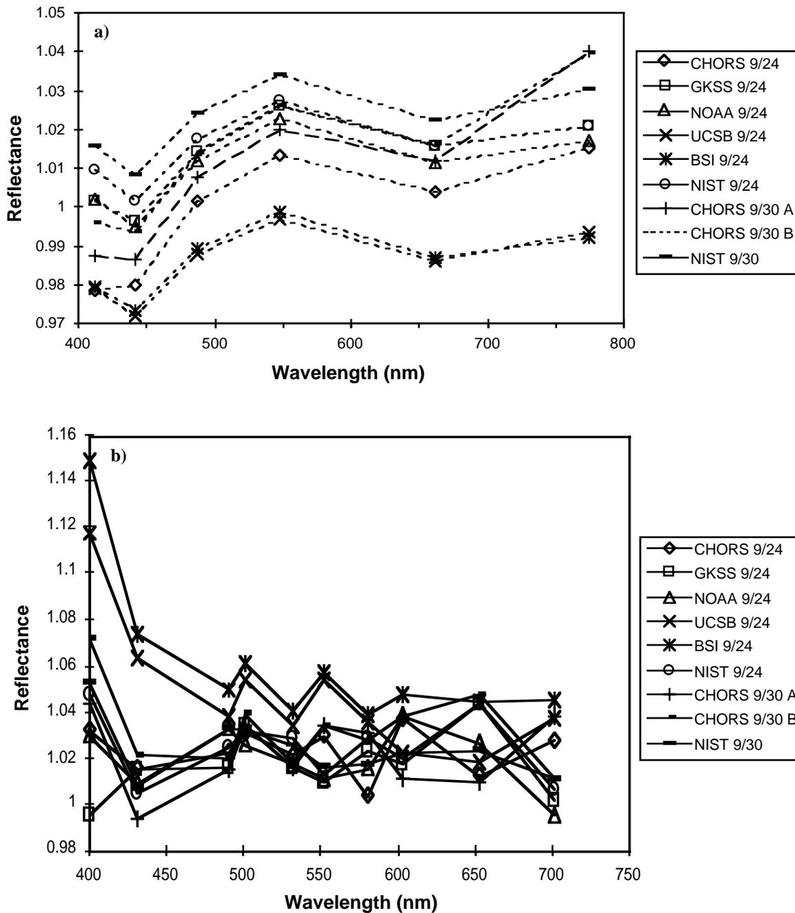
**Fig. 33.** Reflectance factors of all Spectralon plaques (Table A-1) estimated from radiance measurements by the SXR (panel a) and the CXR (panel b) at a viewing angle of  $45^\circ$ . The plaques were illuminated with FEL lamp H91534 at normal incidence at a distance of 150 cm (148 cm for the UCSB and the BSI plaques). The SIRREX-3 values for spectral irradiance for H91534 (Table 6) was used to calculate the irradiance at the surface of the plaque.
