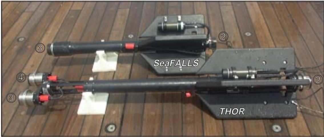
**Fig. 5.** A side-by-side comparison of the free-falling profilers discussed in this report: THOR (front) and SeaFALLS (back). THOR is 1.78 m long and SeaFALLS is 1.24 m long. The numbered bullets on the sensors correspond to the same bullets in Figs. 3 and 4.
