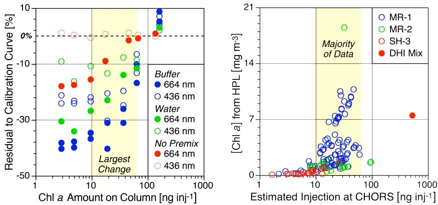
The nonlinearity in CHORS calibrations are reduced if the buffer is replaced by water, and is completely removed at 436 nm if there is no premixing (left plot). The reason the parametric correction is not so negatively influenced by the nonlinearity is the majority of the data—the average response of which almost exclusively influence the parametric correction factors—correspond to the area of largest change in the expression of the nonlinearity (right plot).
