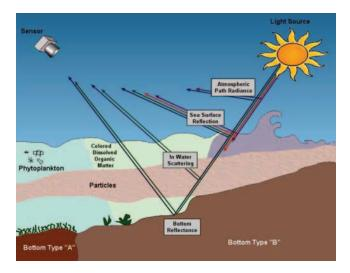
**Figure 1.** Illustration showing the optical complexity found in the coastal ocean, particularly when imaging the bottom. Imaging spectrometer data are required to resolve bathymetry, bottom type and water column optical properties at the same time [1].
