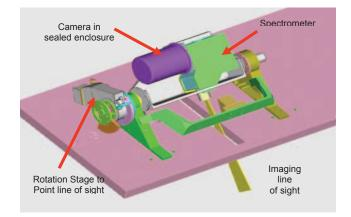
**Figure 3.** An engineering model of HICO. HICO is shown in the imaging position.
