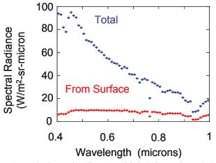
**Figure 2.** Spectral radiance modeled (using MODTRAN) spectral radiance above the atmosphere for 5% surface albedo and 45 degree solar zenith angle. In the blue wavelengths, the atmosphere (total minus surface) is significantly brighter than the surface.
