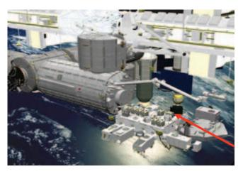
**Figure 4.** The Japanese Experiment Module (JEM) on the International Space Station. The arrow indicates where the HICO and RAIDS Experiment Package (HREP) will be attached to the JEM External Facility.
