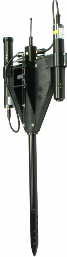
Figure 1: Profiling portion of the Hyperpro system. Ballasted nose-cone at the bottom, E_d radiometer on upper left, L_u radiometer upper right. Between the radiometers are the conductivity and temperature sensors and the power/data conversion unit.
