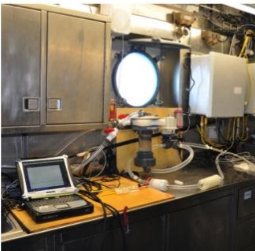
De-bubbling system for the underway IOP cage and tank
