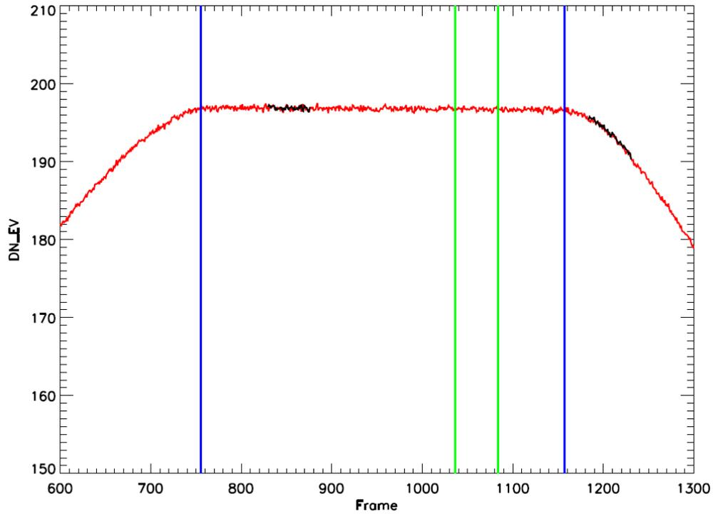
Figure 6: Normalized EV DN for M14 (HAM A, detector 9, SS1, Eside A) with extent of OBC BB plateau (blue) and view (green) shown. Sector rotated BB views are shown in black
