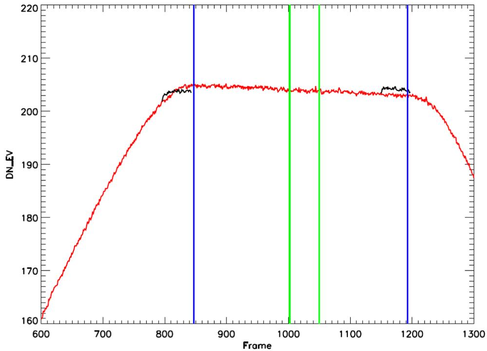
Figure 7: Normalized EV DN for M15 (HAM A, detector 9, SS1, Eside A) with extent of OBC BB plateau (blue) and view (green) shown. Sector rotated BB views are shown in black
