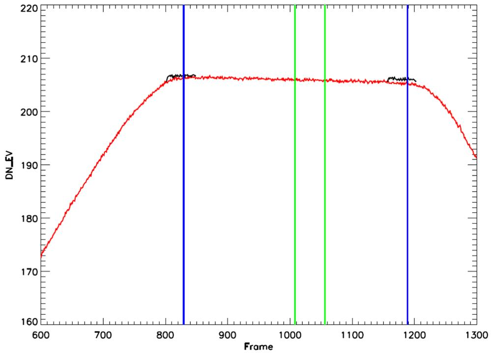
Figure 8: Normalized EV DN for M16 (HAM A, detector 9, SS1, Eside A) with extent of OBC BB plateau (blue) and view (green) shown. Sector rotated BB views are shown in black
