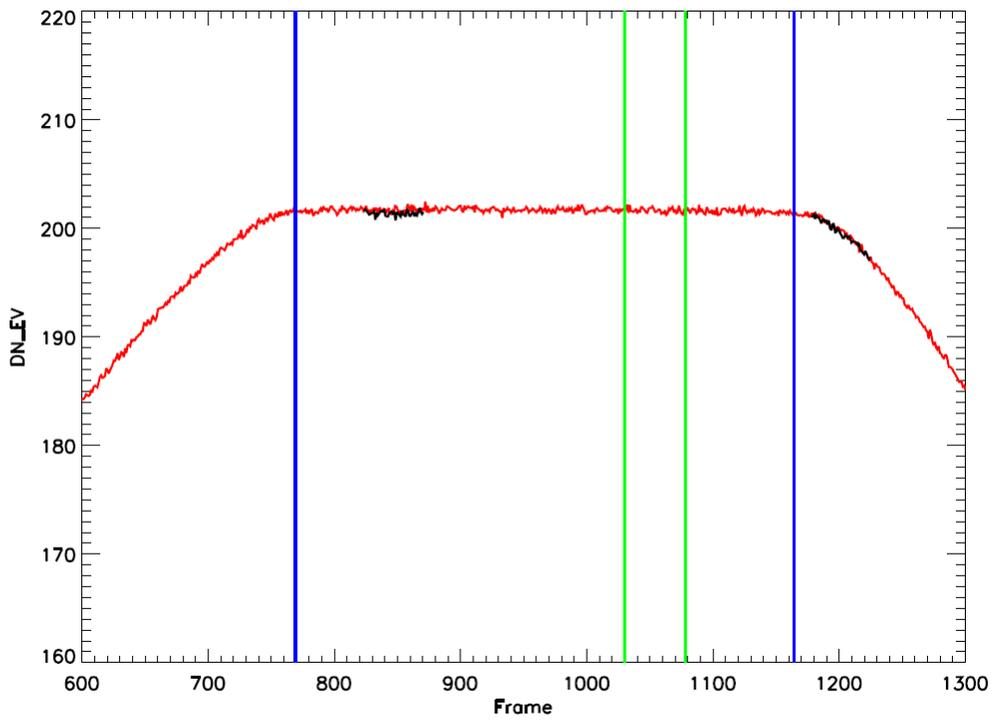
Figure 5: Normalized EV DN for M13 (HAM A, detector 9, SS1, Eside A) with extent of OBC BB plateau (blue) and view (green) shown. Sector rotated BB views are shown in black
