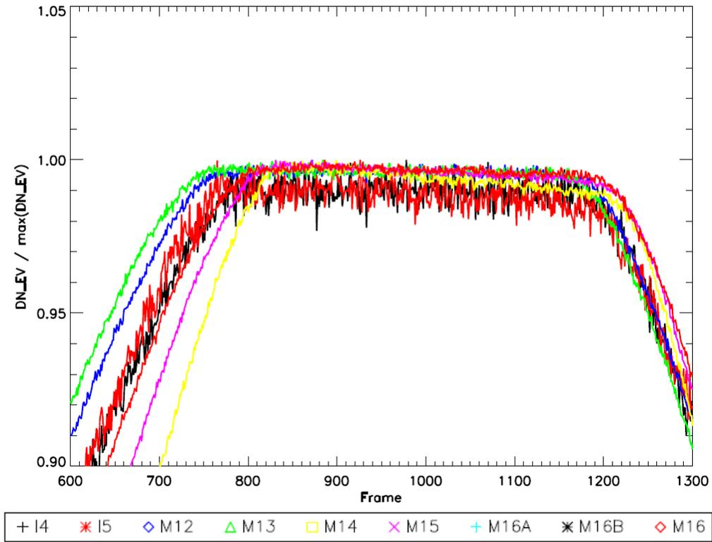
Figure 2: Normalized EV DN for I4 (HAM A, detector 9, SS1, Eside A) with extent of OBC BB plateau (blue) and view (green) shown. Sector rotated BB views are shown in black
