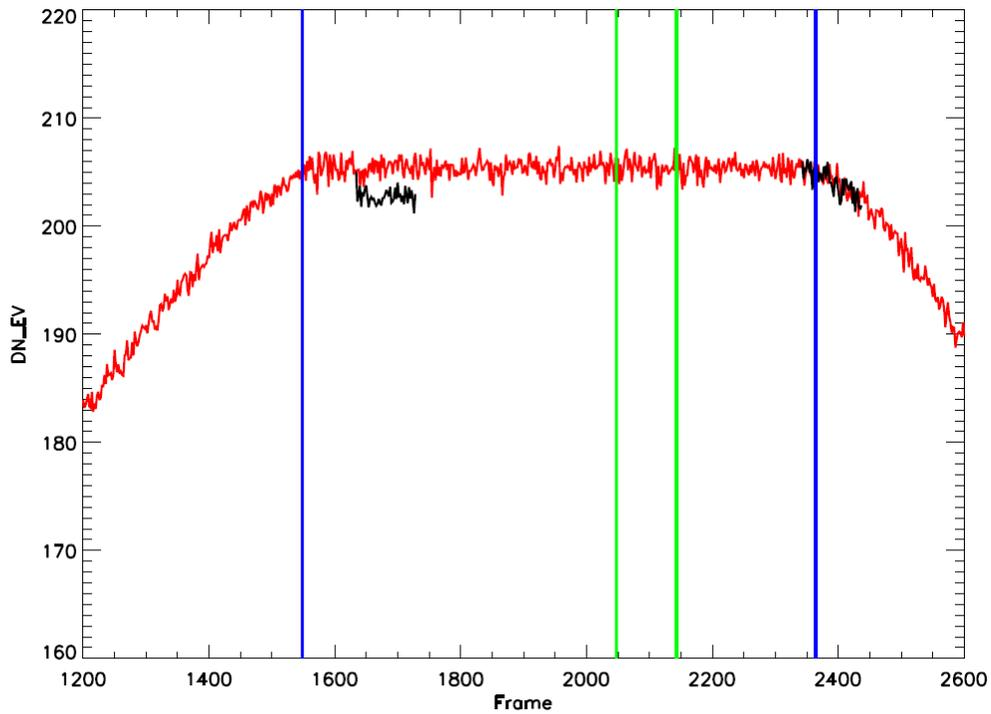
Figure 3: Normalized EV DN for I5 (HAM A, detector 9, SS1, Eside A) with extent of OBC BB plateau (blue) and view (green) shown. Sector rotated BB views are shown in black
