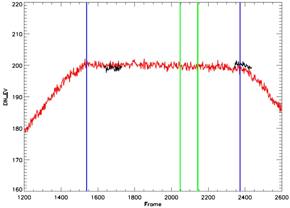
Figure 4: Normalized EV DN for M12 (HAM A, detector 9, SS1, Eside A) with extent of OBC BB plateau (blue) and view (green) shown. Sector rotated BB views are shown in black
