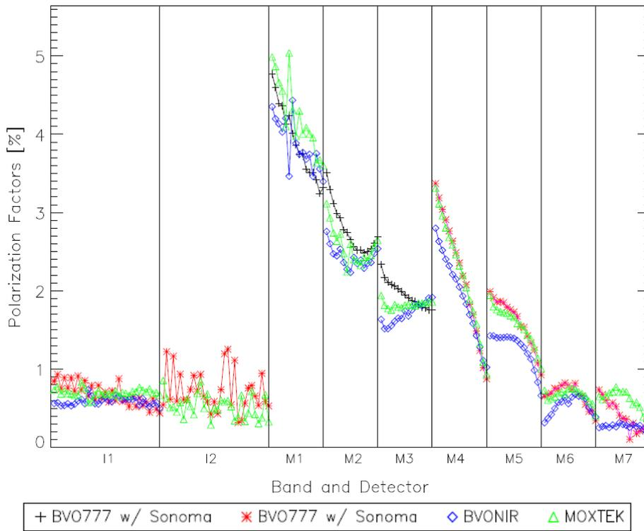
Figure 6: Polarization factor  $a_2$  in [%] for BVO777 test configurations from AOA and sensor level tests
