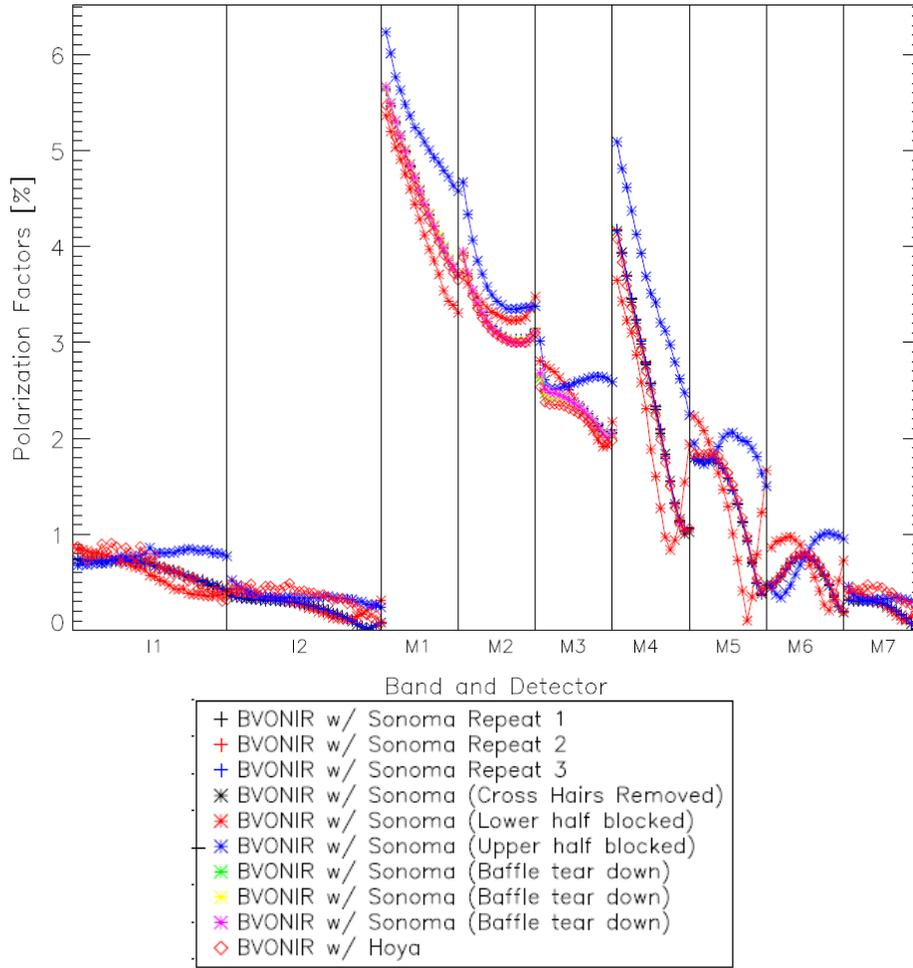
Figure 19: Difference between polarization factors  $a_2$  for HAM side A in [%] between nominal testing and testing using the Hoya filter
