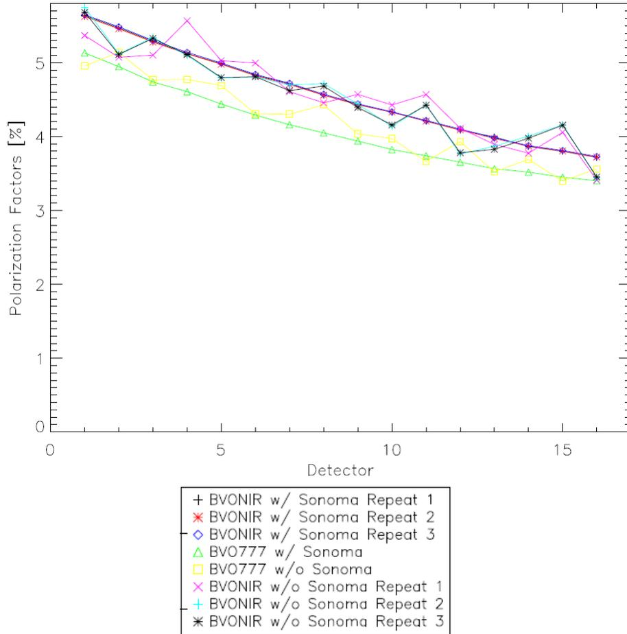
Figure 14: Polarization factor  $a_2$  for HAM side A in [%] across scan angles
