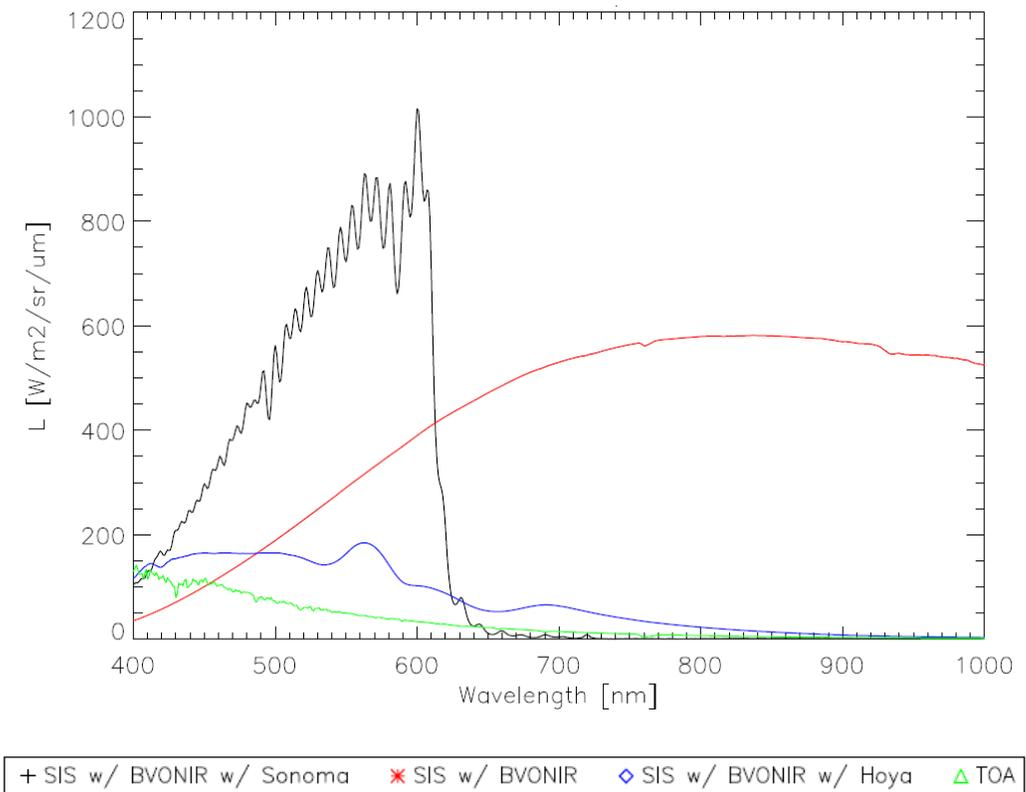
Figure 7: Stray light observed in M7 HAM A using the BVONIR polarizer (no Sonoma filter) with the source dark
