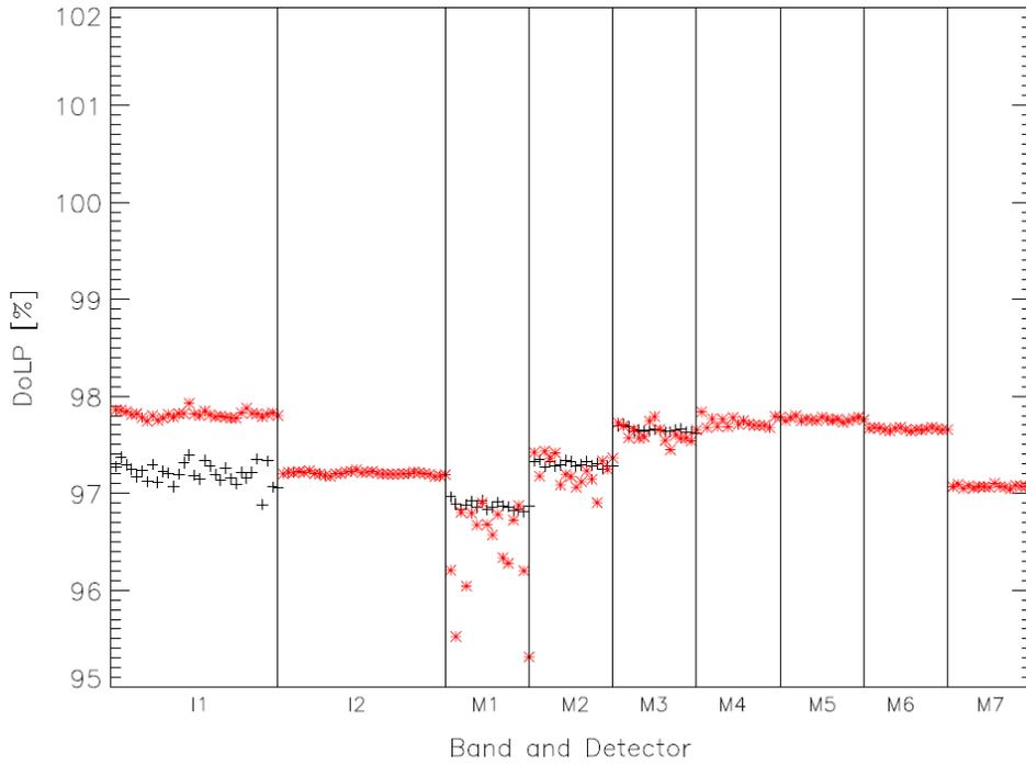
Figure 10: BVO777 polarizer efficiency determined with (black) and without (red) the Sonoma filter
