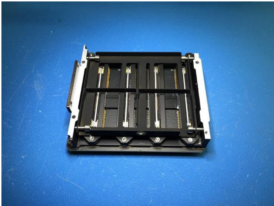
Figure 6: Shutter atop CCDs, in OPEN position. Note – circuit board is painted black, as is most of the CCD ceramic substrate. The vertical silvery stripes are the CCD silicon. Detectors are windowless.
