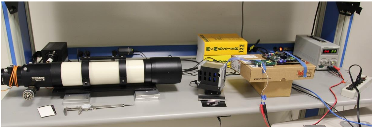
Figure One: Televue Refractor illuminating Instrument on Rotary Stage
