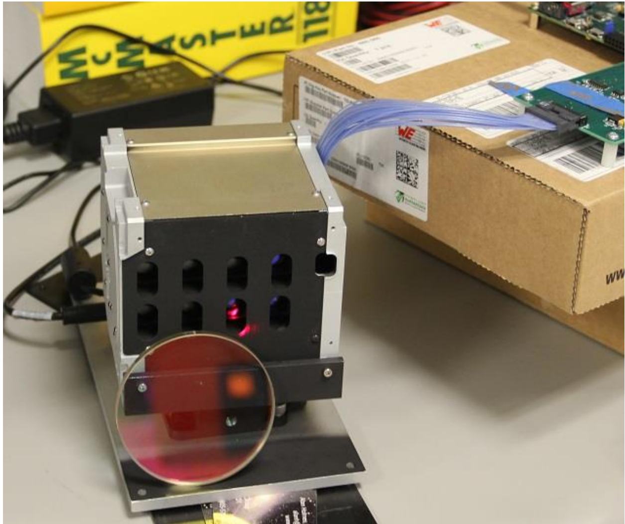
Figure Three: Glass Disk against Instrument Face, Laser Spot on Band 6
