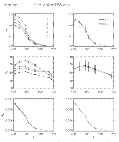
**Figure 4.6** A representative example of how replicate surface spectra measured at a single station are compared with the purpose of assigning a single representative spectrum to the station. Stations are defined using narrow temporal and spatial boundaries.
