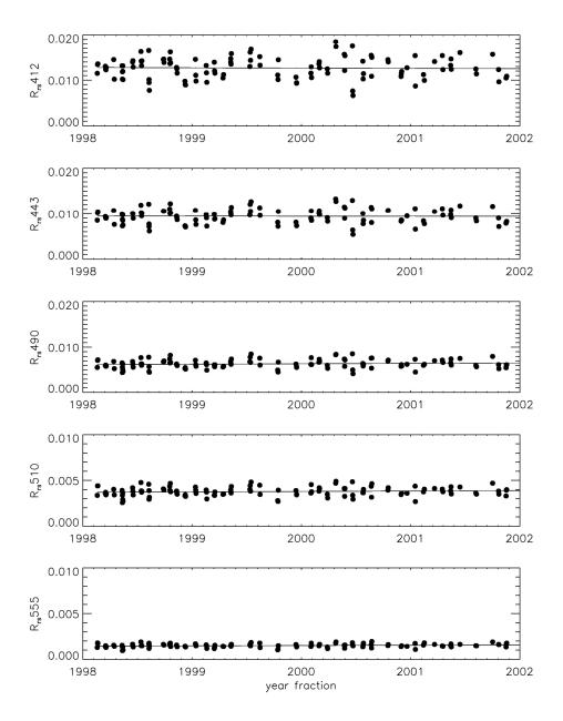
**Figure 4.5** A representative example of a time series analysis of radiometric data, specifically, remote-sensing reflectance, collected on a long-term field campaign. Such analyses are used to help verify the radiometric stability of data archived in SeaBASS.
