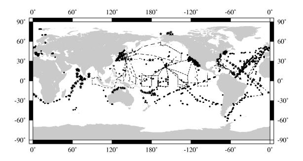
**Figure 1.4** A map of all data points in the SeaBASS atmospheric data set. The locations of MicroTops sun photometer data are indicated with stars, SIMBAD radiometer data with circles, and FRSR data with single points.
