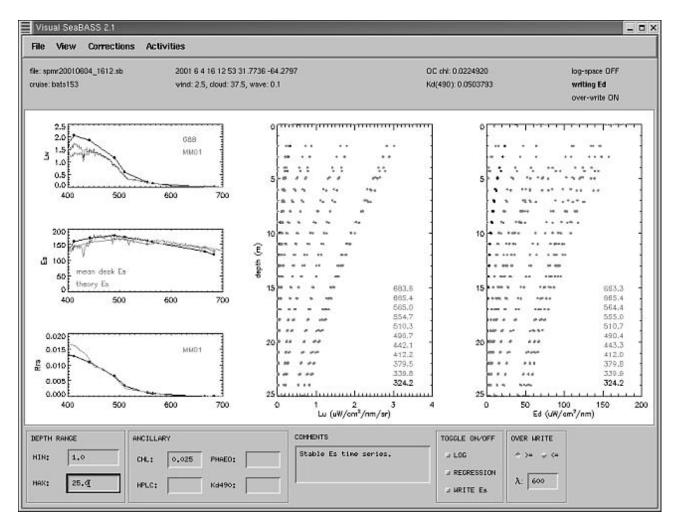
**Figure 4.4** A screen-capture of the interactive software, *Visual SeaBASS*, used by the SPO to evaluate radiometric profiles and prepare data for their satellite validation and algorithm development activities.
