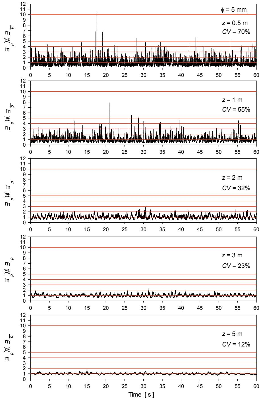
Detailed view of individual wave-focusing events that show very strong pulses of short duration in the  $E_d$  signal
