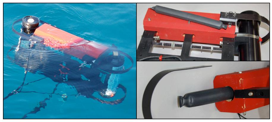
The newest version of SuBOPS uses 19-channel microradiometer sensors. The reduction in weight permits a further improvement in near-surface sampling:
