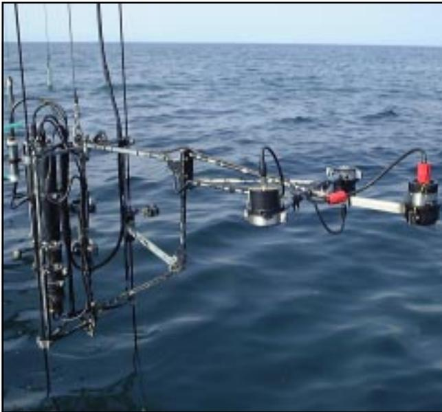
**Fig. 6.** A picture of the WiSPER system immediately before being lowered into the sea.
