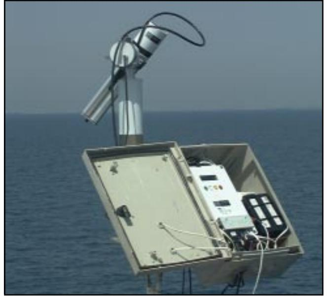
**Fig. 12.** The SeaPRISM instrument being used on the topmost platform of the AAOT. The collimators are the two long tubes pointed towards the sea, and the box in the foreground contains the central processing unit and rechargeable batteries.
