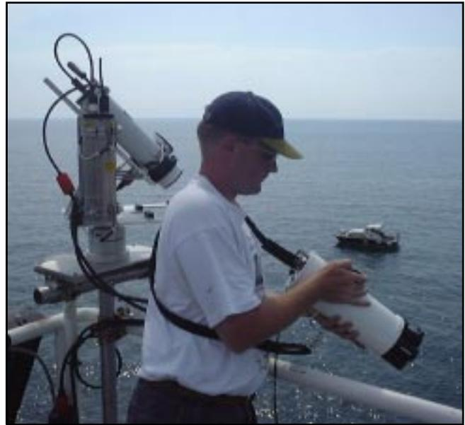
**Fig. 10.** A picture of the handheld SIMBAD instrument being used on the topmost platform of the AAOT (note the SUnSAS instrument in the background).
