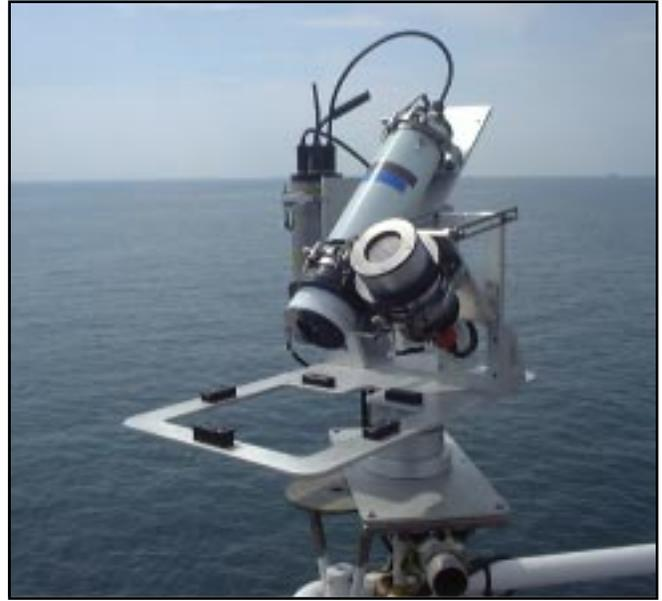
**Fig. 8.** A picture of the SUnSAS frame on the topmost platform of the AAOT showing the square aperture for plaque measurements (not made during the SeaPRISM commissioning) and the two radiometers pointed towards the sea and sky. The cylinder in the background is the DIR-10.
