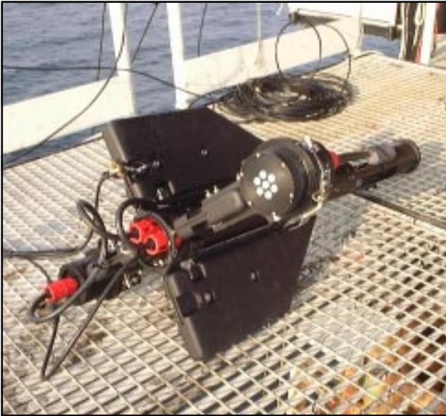
**Fig. 4.** A picture of the miniNESS profiler on the AAOT deployment platform. Note, the platform floor is an open grid which helps reduce the shading effects of the tower, but does not eliminate it.
