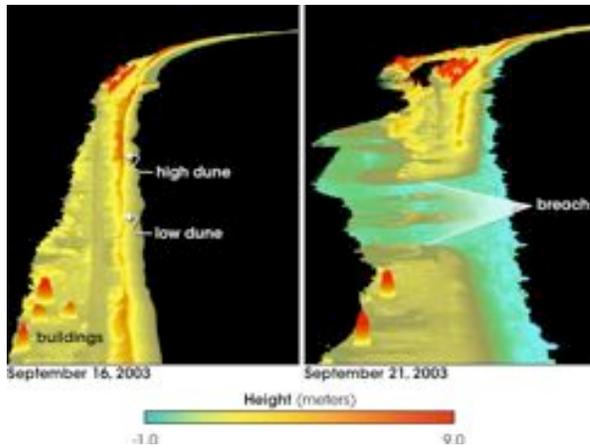
*NASA's Experimental Advanced Airborne Research Lidar shows where sand and buildings on Hatteras Island disappeared in the wake of Hurricane Isabel*
