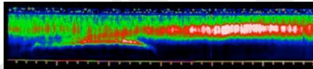
LIDAR track from offshore to onshore, near Wallops Island, VA. Note the entrainment of sediment in the current from the shoal. Courtesy of F. Hoge, <http://aol.wff.nasa.gov/>
