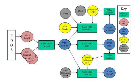
Figure 1 – VIIRS Level-1 Processing Flow
